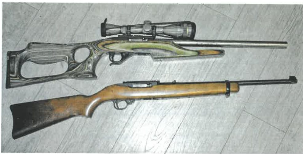
Why have a Plain Jane .22? The top tricked out rifle is the most accurate .22 the author owns. It has a custom made Leupold scope that is painted to match the Boyd's stock, a bull barrel from Brownells and a Timney trigger.
