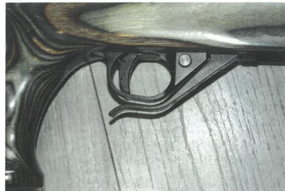
Timney Triggers are the best after market triggers the author has tested. However on this model the magazine release can be in the way when hunting. It's easy to bump and accidentally release the magazine.
